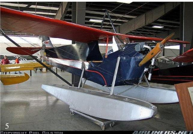
Even with only 36 horsepower some C-3's were flown on floats as shown in picture 5 and 6.
