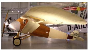
open cockpit is located in the top of the fuselage aft of the wing and offset to the left so the pilot could lean out and peer under the wing for takeoffs and landings. The very wide wing struts were intended to add wing area and lift. Power was from a 90 hp Anzani. This airplane set lots of records for speed and efficiency in the 20s, but the \$5000 price tag scared away buyers. The airplane did lead to a series of later high-wing Bellancas that saw better financial success.
