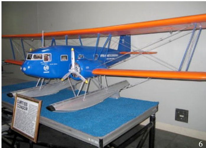
The large Curtiss Condor in picture 6 has a 16 ft. wing span and is powered by two 43 cc gas engines. It is spectacular.
