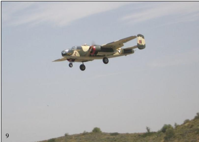
big model built from Ziroli plans with two gas engines and a span of over 100 in. It flew very well. It is on the approach with gear and flaps down in picture 9.
