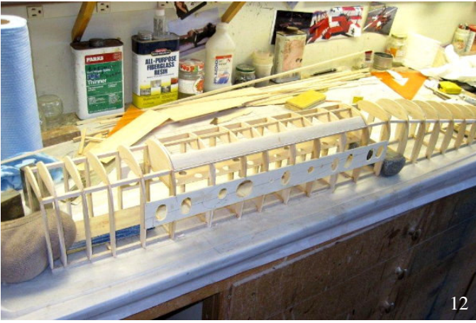
The fuselage started with a flat top to aid initial building as shown in picture 12. Partial formers and some of the aft stringers were added. Then it was turned over and finished.
