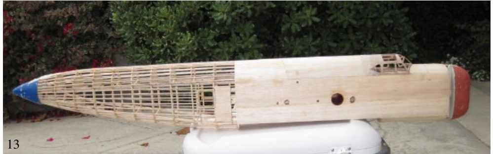
The completed fuselage is shown in picture 13. The front and back ends are all glass (plastic).
