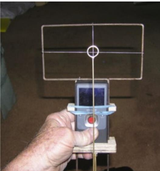
← Put the crosshairs on the airplane, then circle it with the aft reticle and it follows the plane simply with your ability to point it.
