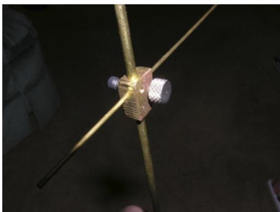
end fits in the square tube on the bottom of the plywood mount and is retained by the thumb screw. Heavier horizontal piece is 1/8" brass rod, lighter vertical piece is 1/16" brass rod with the sighting reticle formed out of 1/16" brass rod around a 3/8" mandrel and soldered to the vertical piece.
