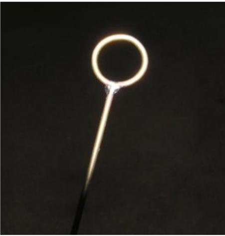
This is the aft sight reticle, 1/16" brass rod loop bent and soldered to the vertical rod.
