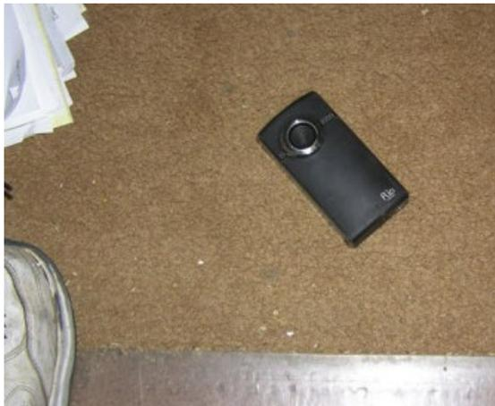
The camera is an HD flip video. It has auto focus, a pretty poor zoom feature, and a backside viewfinder screen. Uses 2 AA batteries and has about 2 hours of video capacity.
